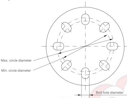
Universal flange (plane flange and Easy Aimer flange) mates with bolt hole pattern of: EN 1092-1 (PN16) ASME B16.5 (150 lb) JIS 2220 (10K)
